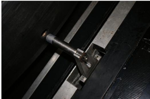
(a) Connection between the dynamometers and the transverse bar. Note the extended slot used to raise the model up, and the tape on the bar. Though it was not possible to fix the model on the bar due to the curvature of the hull, it was an interference fit, and the tape was used to mark the position of the model, confirming it did not travel along the bar during the experiment
