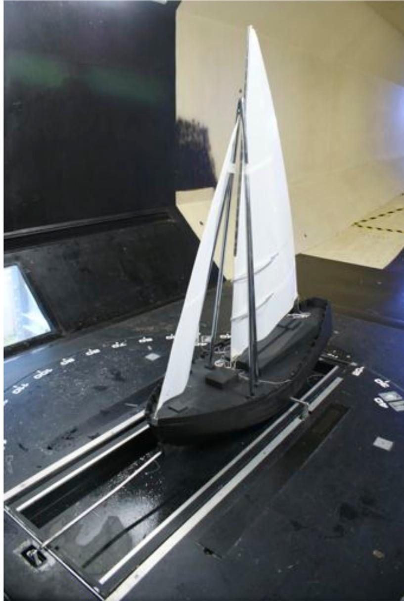
**Figure 37:** *Experimental setup for the physical experiments, upright condition*
