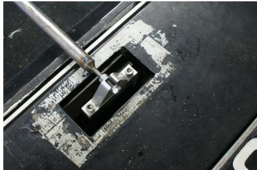
(b) Connection between the bow bar and the flexure. Note the use of an M6 screw thread to enable fine adjustment of the bow bar length
