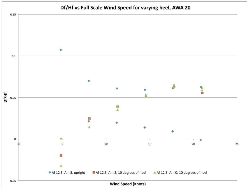
**Figure 65:** Ratio of Drive and Heel Forces against Full Scale Wind Speed in Knots at 10 degrees of heel, with an apparent wind angle of 20 degrees
