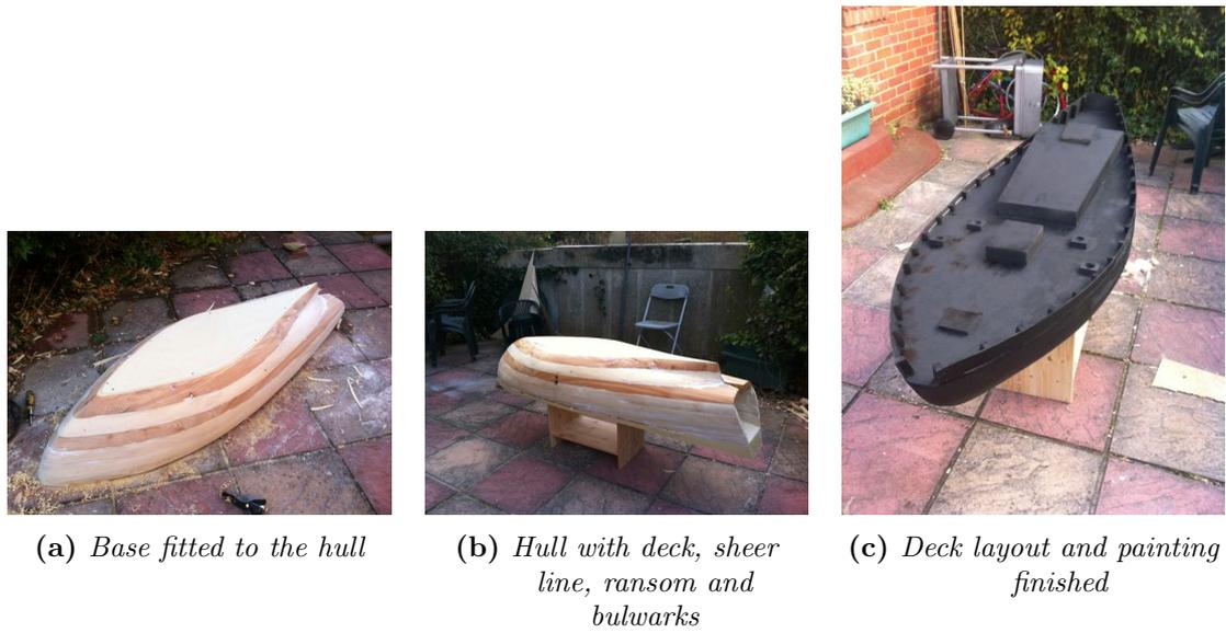
Figure 30: Finishing the hull
