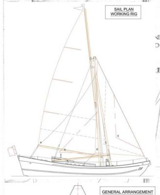
LOA 39'10"/12.1m Beam 12'6"/3.82m Draft 6'9"/2.06m Displacement 16tons
